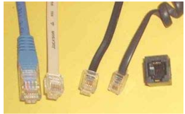
Left to right, modular connectors: 8P8C plug, 6P6C plug, 6P4C, 4P4C, 6P6C Jack
